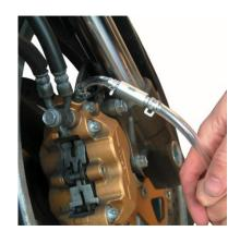
Open (but do not remove) the bleed nipple on the brake calliper.
