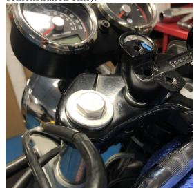
5. Beneath this is a flat solid washer (b), lift this out (sometimes it sticks to the threaded cap).
