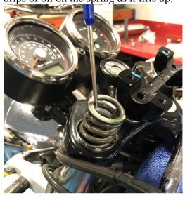
9. Fit the new spring in place with the tighter coils at the top of the fork leg and reassemble the other components in reverse order. This can be repeated for the other fork leg.
