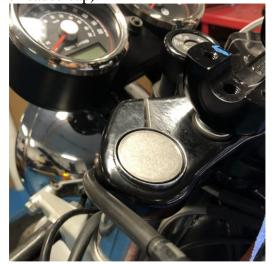
6. The spacer tube (c) is next to come out, a magnetic stick is best for this and simply lifts out.
