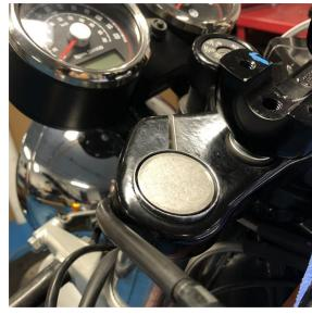
5. The pre loader can now be fitted in place. To make it easier to fit, ensure the centre is unwound to its fullest extent so that the least amount of pressure is applied as it is fitted. The centre of the pre loader uses a standard 12mm bi-hex ring spanner or 12-sided socket, and the outer uses a 27mm spanner / deep socket.
