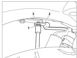
**3** Refit the front grab rail fixing (1). Tighten the fixing (1) to **25 Nm**.
