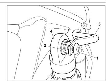
**2** Remove the front grab rail fixing (1) securing the lift handle (2) to the motorcycle frame (3). Remove the lift handle from the motorcycle.
