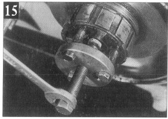
Works Replicas, 500cc Bullets and Enfield's Twins this plate holds the internal clutch cush drive rubbers in their place, though the latter is a luxury not afforded to Roadster 350cc Bullets, or the even more basic 350 Clipper.
