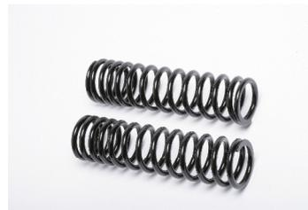
Another option is to fit dual rate springs, available for certain models. These springs give a softer ride and improved road holding. New springs ought to be fitted when the springs have 'set' by more than  $\frac{1}{4}$  inch. Any of these jobs will require dismantling the shock absorber units.
