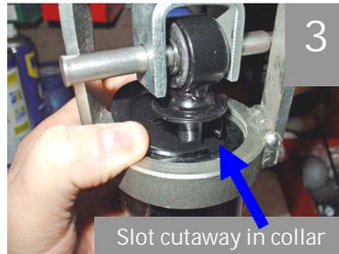
One type of Armstrong style unit uses two springs. These units are a little more complicated than the standard items but the method for dismantling them is the same — once the split collets have been removed the entire unit is easily dismantled.
