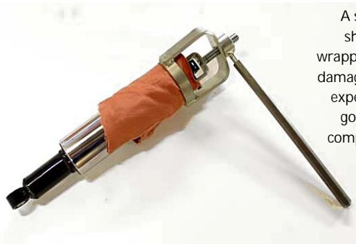
A spring compressor fitted to a shock absorber, showing cloth wrapped round the unit to prevent damage to paintwork. A useful but expensive tool — in most cases a good strong arm will be able to compress the springs sufficiently without this device!
