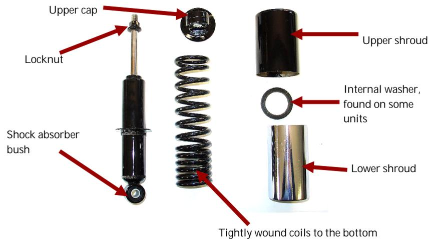
To dismantle these units, a concealed locknut, on the central stud, must first be loosened. The locknut is located under the upper shock absorber shroud, which must be lowered to give access to the locknut.
