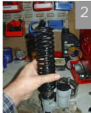
If fitted, the spring covers may be removed, along with the main spring (photo 2).
