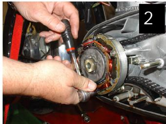
Because the primary drive uses an 'endless' chain, both the engine and clutch sprockets must be withdrawn together with the chain, as one complete assembly. To facilitate this it is necessary to remove the alternator stator and rotor. Remove the stator by undoing the three holding nuts (photo 2) then lift the stator
