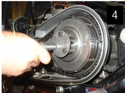
Slacken and remove the three clutch spring pins. Lift away the springs, the outer clutch plate and clutch pad, ensuring that any ball bearing, if fitted, does not drop out of the end of the gearbox mainshaft (photo 4).
