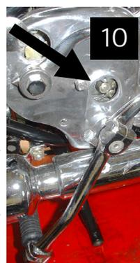
cover and screw. Adjust the cable free play with the cable adjuster, allowing about 5mm free play at the lever. Take
