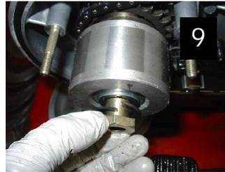
Before replacing the clutch plates, take time to check that the plates are perfectly flat using a straight edge and the friction plates have a working thickness of friction material (the friction discs when new are approx 4.5—4.7mm thick). Clean the discs (carb cleaner is an ideal choice for this) then replace in the correct order, the reverse order in which they were removed.
