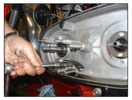
STEP 4: Undo the nut holding the primary chain tensioner and slide the tensioner off. The clutch centre with sprocket, engine sprocket and chain will now slide off their splines as an assembly. If the engine sprocket is tight on its shaft use the special engine sprocket extractor tool (ST25098).
