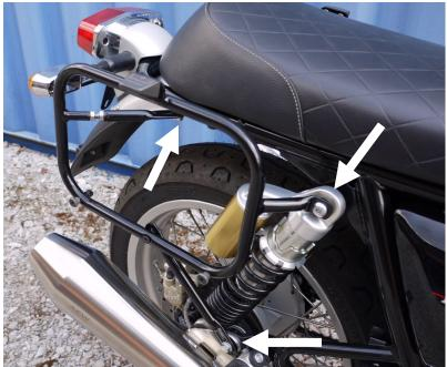
Loosely fit the top front fixing of the pannier frame mount to the rear shock absorber top bolt using the existing bolt. Please note: The rear shock absorber top bolt can be loctited in at the factory and it is important to use a well-fitting Allen Key to prevent rounding the head of the bolt.
