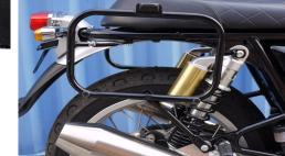
The rear adjustable arm attaches to the rear most hole on the underside of the seat frame where the grab rail is bolted. Use the existing bolts, but do not tighten yet. The pannier frames will fit with or without the grab rail.
