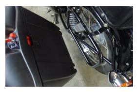
Drop the pannier box down onto the lower mushrooms then push the upper part of the pannier box towards the top lock clip. It should click into position.
