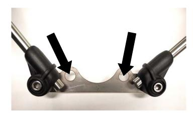
3. Assemble the two brackets around the handlebars using the two <u>straight</u> metal rods and the half circular 'pads' to protect the handlebars. The <u>straight</u> rod will eventually attach to the brackets identified in step 4 of these instructions.
