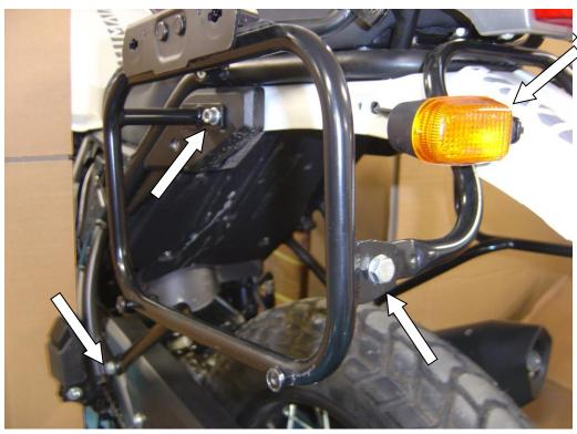
You will now need to reposition the rear indicators onto the side frames. Remove the 3 x 10mm nuts and 2 x 4mm Hex screws on the liner underneath the mudguard in order to release the indicator cables from their block connectors.
