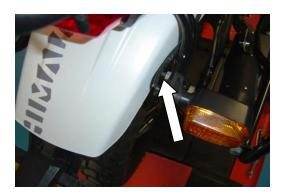
Insert 2 of the Lower Fixing Mushrooms using 2 of the Black Hex Socket Screws M6 40mm and 2 of the M6 Nuts Nyloc Black into the bottom of each side Pannier Frame (SEE PHOTO ABOVE LEFT) which will be used to secure the side Panniers
