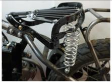
Saddle and springs bolted in place. Note the positioning of front securing bolt and how the springs are attached.
