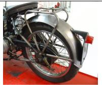
Saddle, carrier, mudguard, number plate holder and tail light bolted in place.
