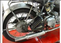
Toolbox bolted in place and exhaust reinstalled.
