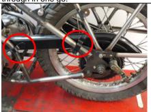
Chainguard fitted. It attaches in two places (circled).
