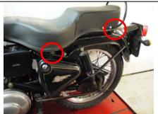
Remove the seat by removing the bolts each side as circled.
