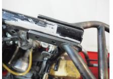
Subframe top section lined up with main frame (attach subframe via it's lower mounting points first).
