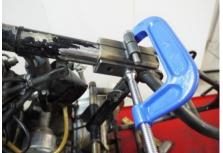
Clamp the fixing plates to the main tube to prevent movement while drilling.
