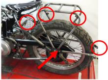
The rear carrier is secured to the sub frame by a single bolt on each side (arrowed). The carrier is then secured to the mudguard by means of the lugs and supports as circled.
