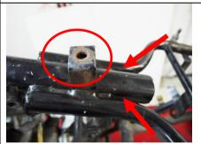
Cut this bracket off first, to provide more room for cutting through the frame loop welds on both sides (arrowed).
