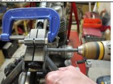
Drilling the final holes (10mm drill). Do each side separately. Don't drill right through in one go.
