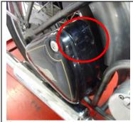
If your ingition switch was mounted in the LH toolbox, you will need to relocate it to the RH one. Drill a suitable size hole in the area circled.
