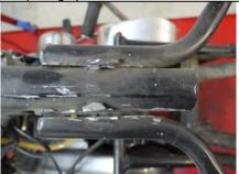
Frame welds successfully cut through.
