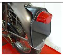
Mudguard attached, drilled and number plate bolted in place.
