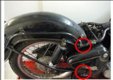
Disconnect the tail light wiring loom. Remove the mudguard and frame complete, by undoing the retaining bolts and pulling up and rearwards.
