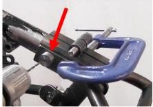
Use the small pilot bush (arrowed) to drill a 3mm pilot hole. Do each side separately to ensure hole accuracy.
