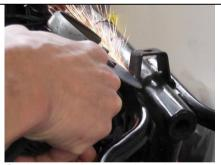
Cutting through the bracket prior to cutting through the welds between the main tube and the sub frame loops.
