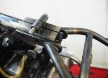
Fixing plates correctly positioned. Push a bolt through the top lugs to hold the plates in position.
