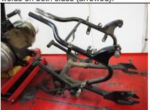
Old subframe removed (shocks, wheel, toolboxes and chainguard taken off first to lighten it).
