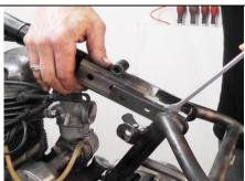
Slide the subframe fixing plates into place. You may have to apply some gentle leverage and tap into position.
