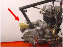
To prevent the frame down tube dropping, after the rear frame is removed, wedge a wooden block on top of the gearbox (arrowed).
