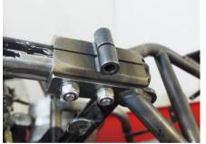
Holes drilled and fixing plates securely bolted in place.
