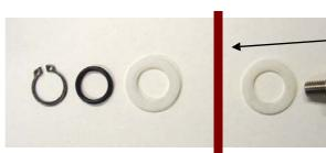
The tool box lid will be positioned here – between 2 nylon washers
