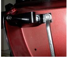
located in the threaded hole, tighten the bolt securing the bracket in the tool box. The ring spanner you left inside the tool box will allow you to tighten the bolt firmly from outside the tool box.
