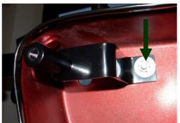
Assemble the thumb screw components in the tool box lid, in the order shown above. At this stage *do not* secure them with the circlip.
