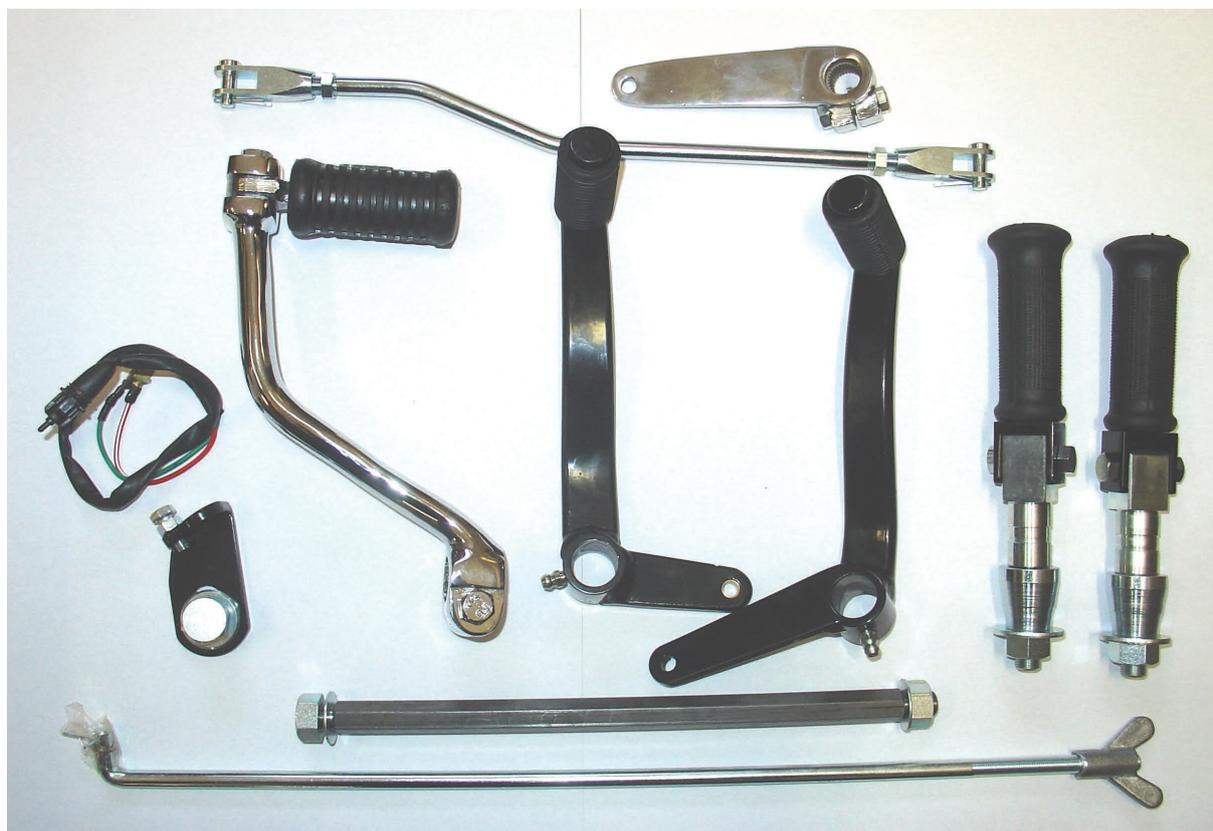
This Rear set kit is designed to fit and work with the Hitchcock's Café Racer kit. It will be assumed that the rest of the kit has been or is in the process of being fitted, and that all necessary original parts have already been removed including footrests, pedals, exhaust systems etc.
