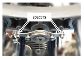
2. Loosely fit the frame bracket to the frame with the supplied M6 socket head screws, washers and M6 nuts. Using the supplied M6 button head screw, washers and M6 nut secure these two brackets together. So they are flush. It may be necessary to alter the angles of the brackets. Fully tighten all fixings.
