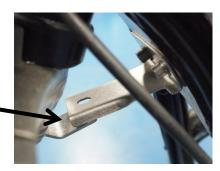
3. Replace steering column chrome nut with newly supplied steering column nut. Fit spring washer to damper rod and insert damper rod through column – screw damper rod until required damping effect is achieved.
