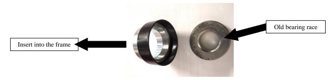
5. Fit the upper bearing race into the frame using the old bearing race as a drift.
