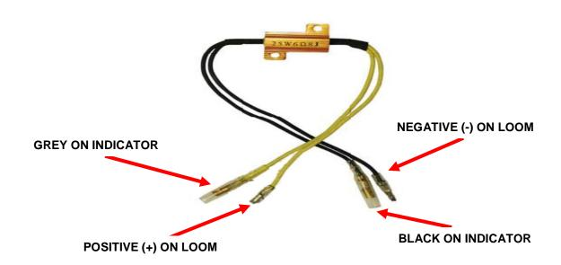
Please note that if you are fitting L.E.D indicators to the just the rear of your Bullet, depending on the model you would not normally require resistors but may require a different flasher unit, part no 92292 which can be ordered separately.
