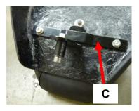
**9.** Front seat bracket (C) hooks under the front attachment bracket (A) like this.
