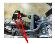
**8.** Fit seat by pushing front seat bracket onto front frame bracket (A) and move rear bracket until the seat bolts fit into bracket holes (arrowed). Push seat fully forward and tighten all bolts.
