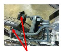
**7.** Attach rear seat bracket to the rear shock absorber bolts as arrowed.
