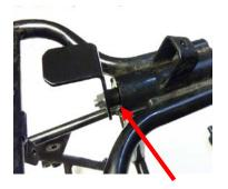
**4.** Push the rubber bush fully into the top frame tube and turn the nut to expand the bush.
