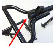
**3.** Front attachment bracket (A) is inserted into frame top tube (arrow) and secured by an expanding rubber bush (B).
