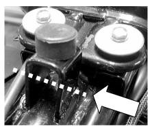
1. Using two nuts and washers attach front mounting bracket to the two studs located at the front underside of the seat.
