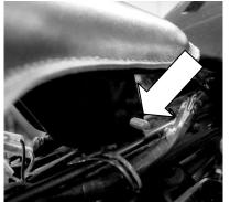
seat may now be bolted to the drilled frame bracket — arrowed. Use the supplied seat bolt to attach the seat front mounting to the frame bracket. Secure with M8 nyloc bolt and washer supplied with the seat. NOTE: do not fully tighten the front mounting bolt — the sprung seat will pivot on this mounting bolt.
