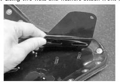
2. Do not at this stage fully tighten nuts on studs to allow fore and aft adjustment of mounting plate — arrowed.
