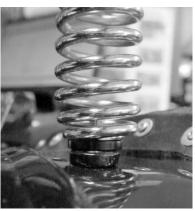
4. Remove nuts from rear frame studs and locate spring loops over studs using special nuts 91403D and special D washer 91403H — see photos below. NOTE: springs are asymmetrical — to 'centre' seat mount one spring with loop <u>forward</u> and one <u>backwards</u>.
