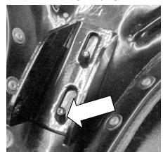
3. Fit the spring mounting stud to the fixing points in the underside of the new seat - shorter stud thread into seat base. NOTE: there are three fixing points for the stud on the underside of the seat — as in photo. Use the forward-most fixing point for E5 and Electra X models.
