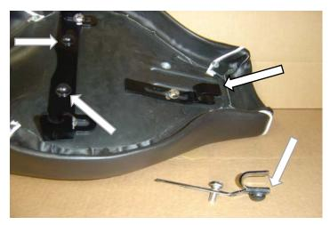
Finally re-fit and secure the seat to the bike using the original nuts and bolts and the remaining 2 M8 x 20mm bolts, 2 flat washers x 5/16ths and 2 Nyloc M8 Nuts and use to secure the rear seat bracket to the bike
