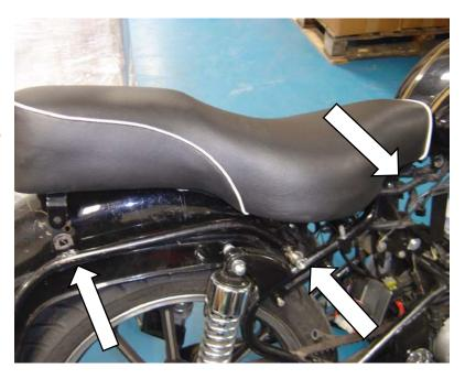
Once you are satisfied with the final fit remove the seat and tighten all brackets on the underside of the seat. Position 2 of the rubber self-adhesive spacers onto the middle seat bracket so that they line up with the top curve of the mudguard. The remaining two are fitted onto the bottom of the two u shaped forks on the front seat mounting brackets (SEE PHOTO BELOW) to provide a buffer between the seat and the frame
