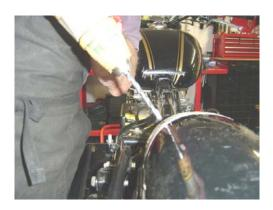
Once the holes are drilled re-mount the rear bracket onto the seat and tighten all bolts (front tongue bolt should already be tight). The seat can now be fitted onto the centre bracket and with the flanged nuts and bolts supplied to the rear one.
