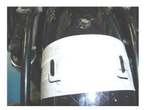
Steps 6 & 7 show position to drill in the middle of the slot and drill angle. Drill size is 6.5mm or 7mm.
