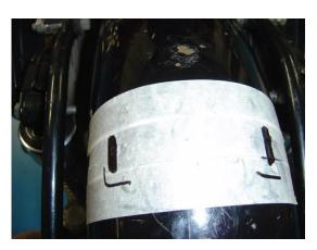
Steps 6 & 7 show position to drill in the middle of the slot and drill angle. Drill size is 6.5mm or 7mm.
