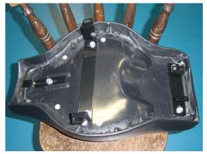
Step 2. Apply masking tape for marking drill points for rear mounting bracket
