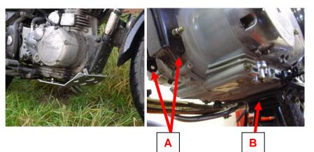
L shaped front brackets attach here (A).
